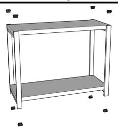
Insert the 8 plastic plugs included in the package by hitting the upper and lower parts of the metal legs with a hard object.
