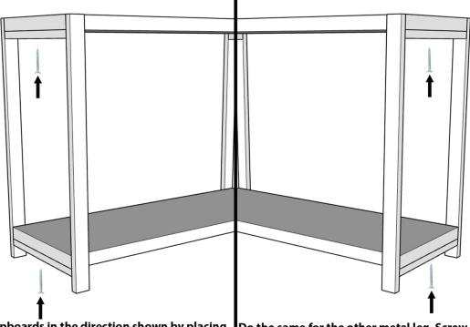
Screw the chipboards in the direction shown by placing them on the metal feet so that there is no gap as seen in the image.
