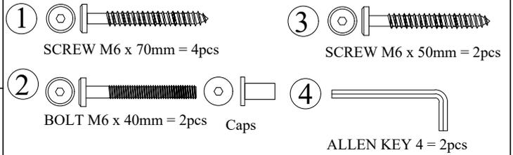
These instructions must be used to ease the assembly of your furniture. Please ensure that you have all the components before assembly. Remember to place the part on a carpeted floor or blanket in order to protect them from damage while you assemble.
