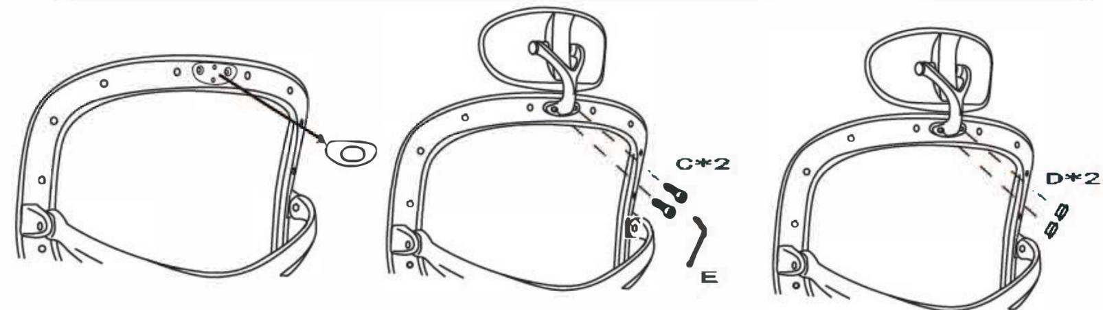
Insert and loosely tighten all screws. When assembly is completed, fully tighten all screws before using. This chair is only intended for sitting. Any other use will void the warranty.
